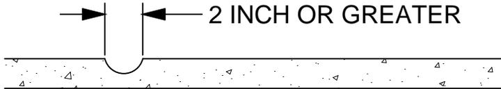
Missing concrete greater than two inches in any direction and/or severe pitting of more than 25% of the flag that causes a bumpy or uneven surface. Deteriorated control joints creating a crevasse greater than two inches in width.
